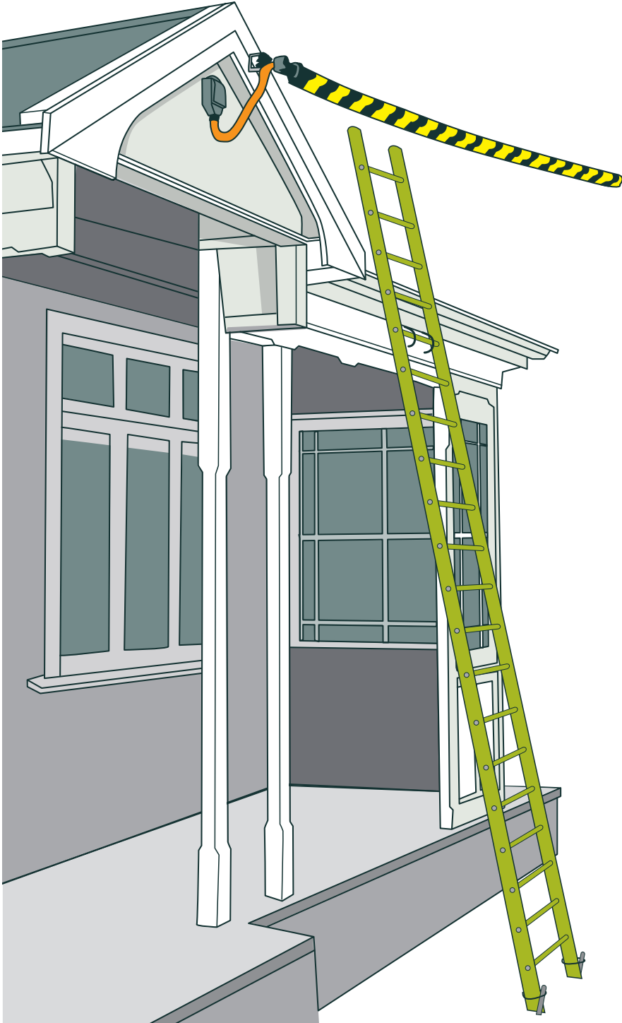
FIGURE 6: Tiger tail on an overhead line
